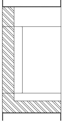
WHEN LINER IS LOCATED IN FORM AS ABOVE, SHIFT THE TOP RECESS TO THE LEFT AND LOCATE THE LIFT BLOCKOUT WHERE SHOWN BELOW
