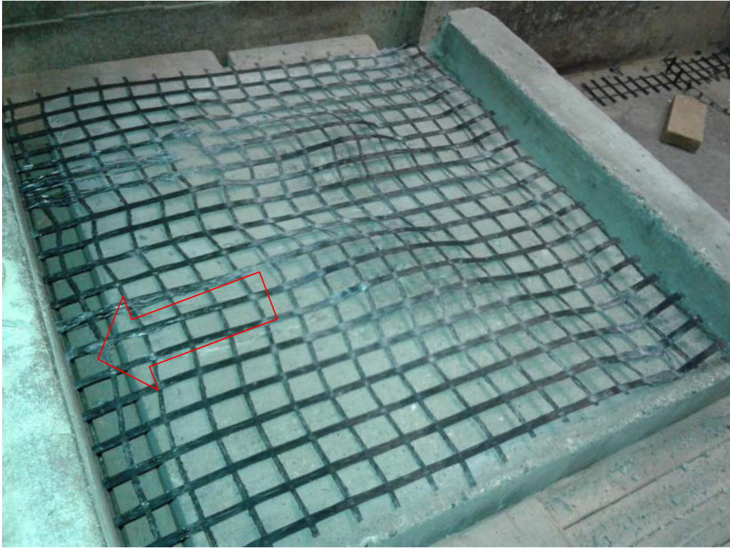
Figure A-4. Abrasion and rupture of geogrid at the completion of a test. The arrow points to direction of connection load.
