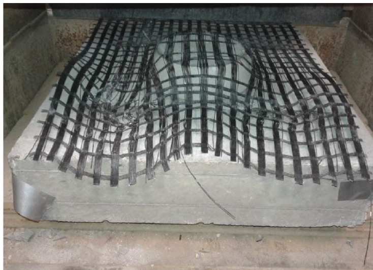
Figure A-4. Abrasion and rupture of geogrid ribs at the completion of a test.
